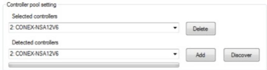
After a *Discover* action, the list of detected controllers is filled. Stage model number is shown next to the address #1 through #4. This address helps to identify each controller connected.
